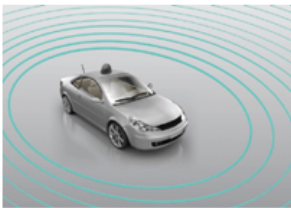
LEFT: FMCW LiDAR sensors generate 360° views around a vehicle.
