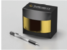
Insight Lidar's frequency-modulated, continuous-wave (FMCW) system.
